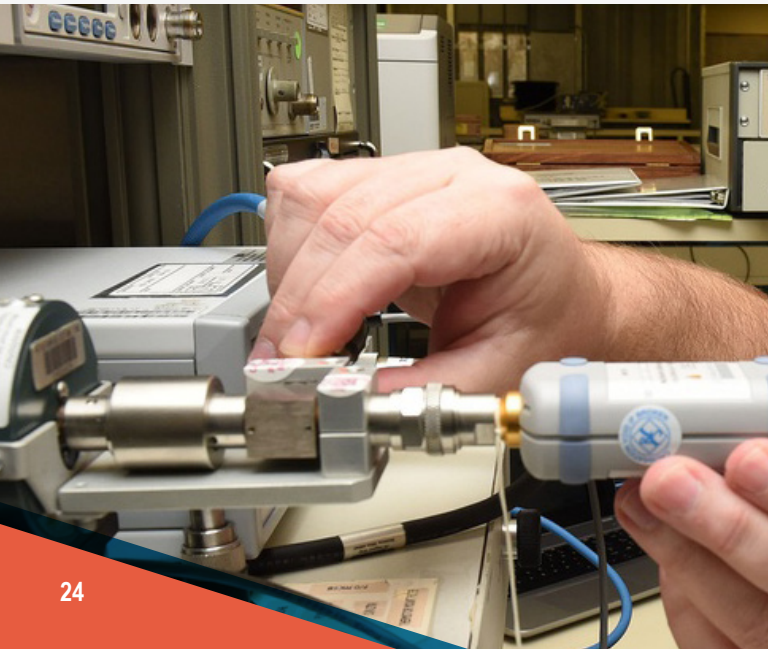
88th Logistics Readiness Squadron precision measurement equipment laboratory lead technician mounts a power sensor on a splitter for calibration test reading. Photo Source: Michelle Gigante, 2017, DVIDS.
